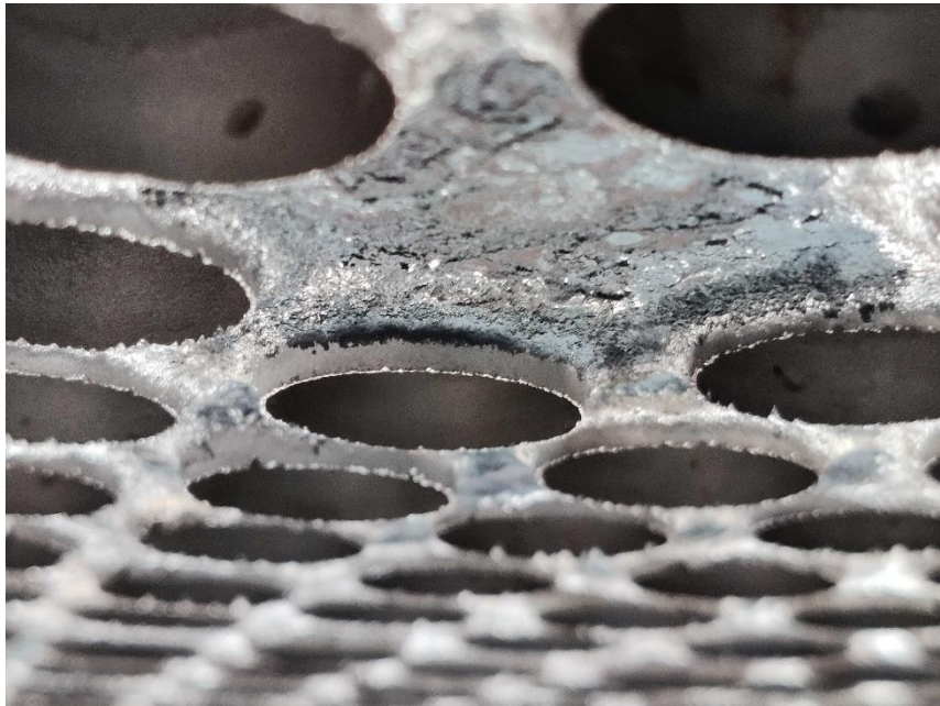
FIGURE 6: THE BOTTOM TUBESHEET SURFACE IN THE CORRODED CONDITION
